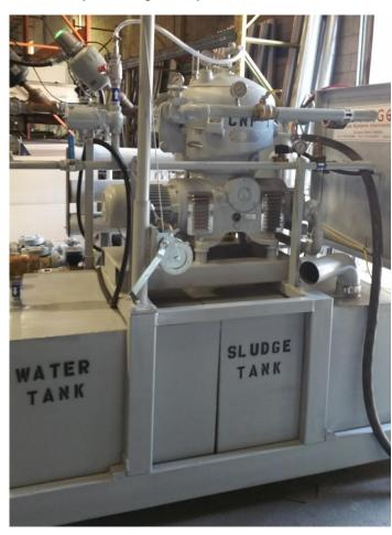
The high-speed centrifuge system typically produces more than 10000G and all modern units are auto-dumping. Liquid-liquid or liquid-liquid-solid separators are available in order to handle sludge or solid particulate contamination usually found in lubrication oil applications.
